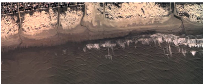
Fig. 14. Wave attenuation and lateral variability in breaker height, surf-zone width and set up associated with presence of mud.
