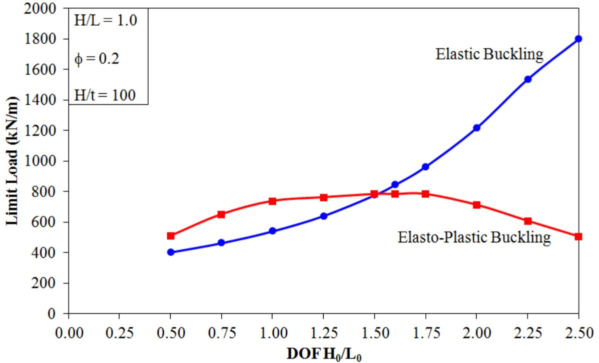
Figure 5. Limit load variation for plate  $H/L = 1.0$  and  $H/t = 100$  as function of the DOF  $H_0/L_0$
