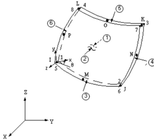
Figure 4. SHELL93 finite element
