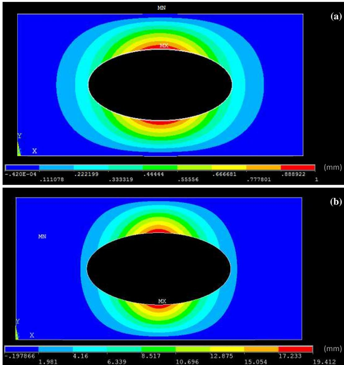
Figure 8. Buckled shape for plate  $H/L = 0.5$ ,  $H/t = 50$  and  $H_0/L_0 = 0.50$  for (a) elastic behavior; (b) elasto-plastic behavior.
