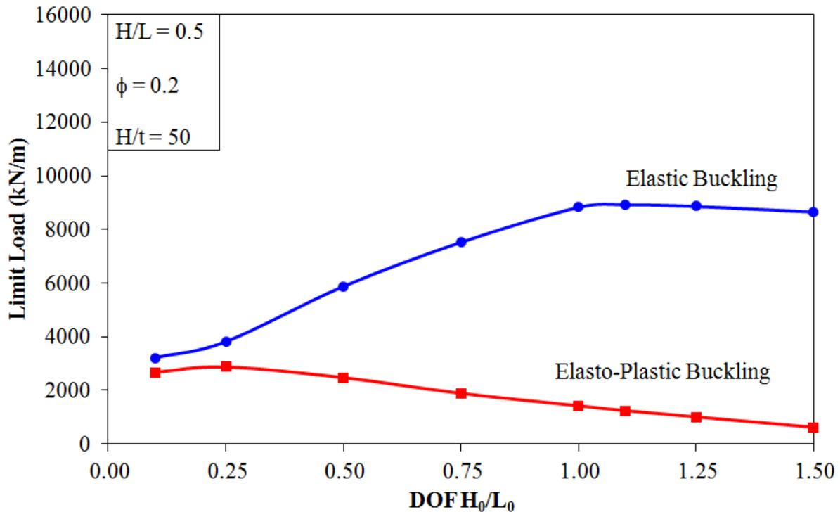
Figure 9. Limit load variation for plate  $H/L = 0.5$  and  $H/t = 50$  as function of the DOF  $H_0/L_0$
