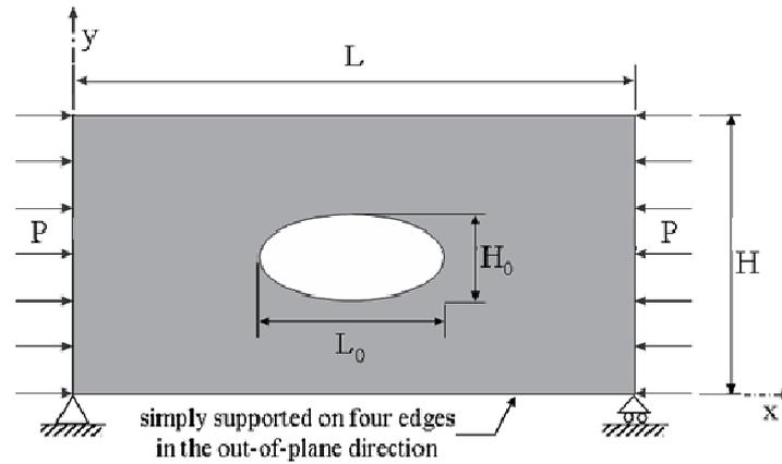
**Figure 1. Geometry and loading of a plate with elliptical**
