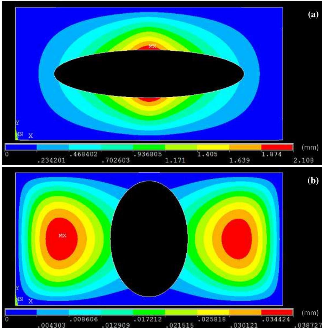
Figure 10. Nonlinear buckled shape for plate  $H/L = 0.5$ ,  $H/t = 50$  and: (a)  $H_0/L_0 = 0.25$ ; (b)  $H_0/L_0 = 1.50$
