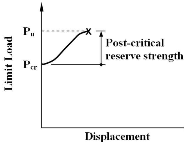
Figure 2. Load/displacement diagram in the post-critical range
