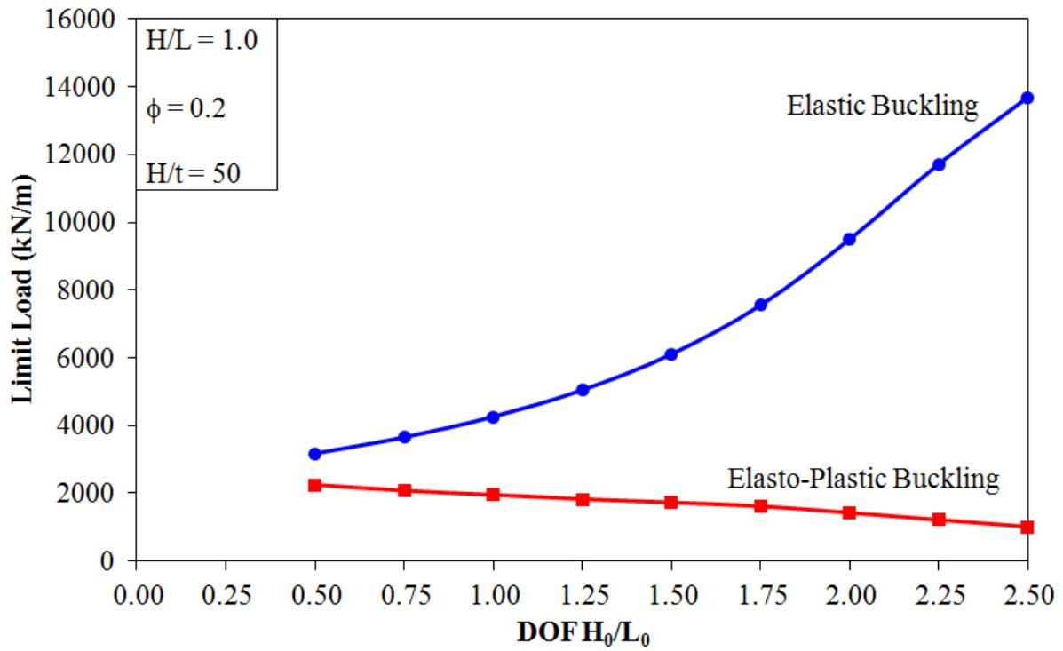
Figure 6. Limit load variation for plate  $H/L = 1.0$  and  $H/t = 50$  as function of the DOF  $H_0/L_0$
