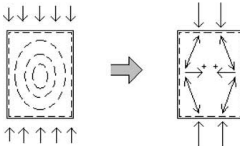
Figure 3. The redistribution of the transfer of load in the ultimate limit state (Åkesson, 2007)
