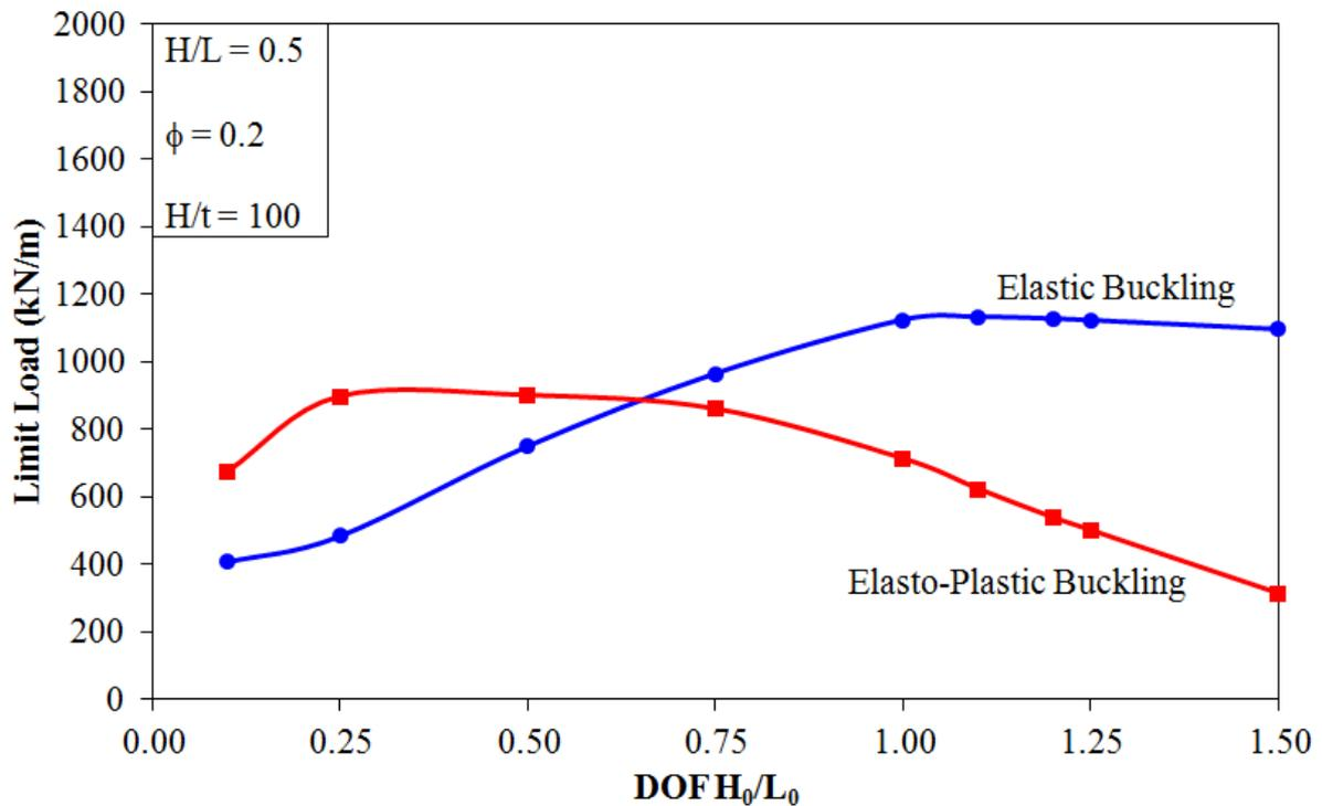
Figure 7. Limit load variation for plate  $H/L = 0.5$  and  $H/t = 100$  as function of the DOF  $H_0/L_0$
