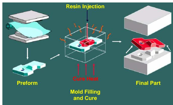
Figure 2. RTM process.
