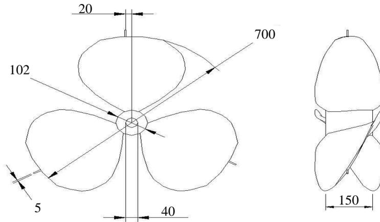
Figure 3. Marine propeller geometry and its main dimensions (in mm).
