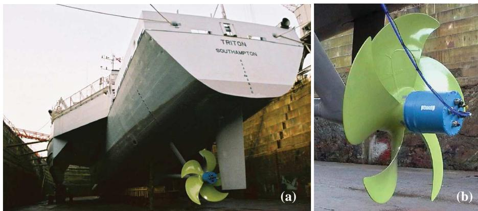
Figure 1. Polymeric composite marine propeller (Marsh, 2004): (a) overview and (b) detail.
