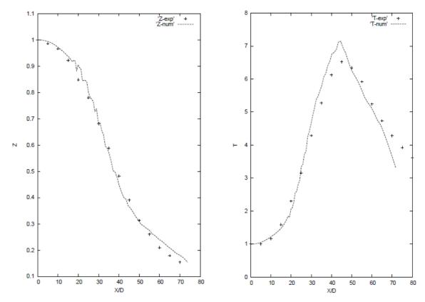
FIGURE 2. Comparison with experimental data [1] for the mixture fraction (left) and temperature (right) profiles along the burner centerline.
