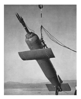
Fig. 2.2: The towed paravane used by Grant et al. (1962) to obtain the first records of micro-scale turbulence in history.
