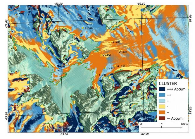
Figure 14: Cluster classification that was conducted with the averaged sigma SAR image and terrain products as input and six classes. The colour code is the relative accumulation rate between areas and is set as the previous classification. Compared to the previous classification, a broader and homogeneous zone of lower accumulation (orange) existed in the central valley downward from the BIA, including SP1 and SP4. The red class is restricted to specific areas close to the mountain.
