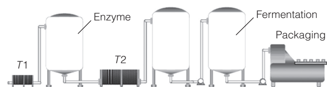
Figure 1. Two-stage lactose conversion process for fermented milks: enzymatic catalysis and fermentation. Source: Martins (2009).
