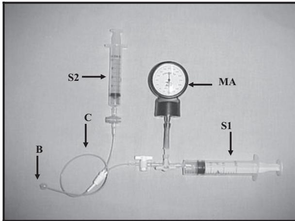
**Figure 1** The burst pressure test system. B, ballonet; C, catheter 2-way; MA, manometer; S1, syringe 20 mL; S2, syringe 10 mL.
