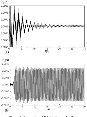
Figure 3. Drag (a) and lift (b) forces for fixed cylinder with Re=105.
