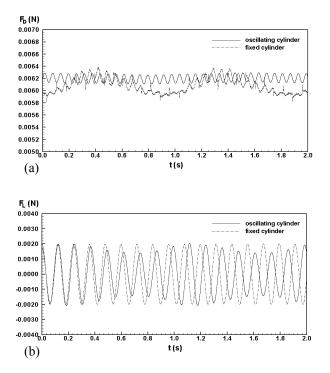
Figure 10. Drag (a) and lift (b) forces for cylinder with Re=123.
