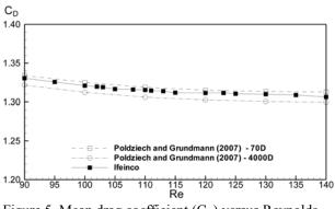
Figure 5. Mean drag coefficient (C<sub>D</sub>) versus Reynolds numbers.
