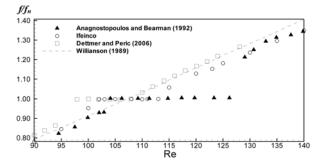
Figure 8. Frequency of vibration (f/fn) versus Reynolds numbers.
