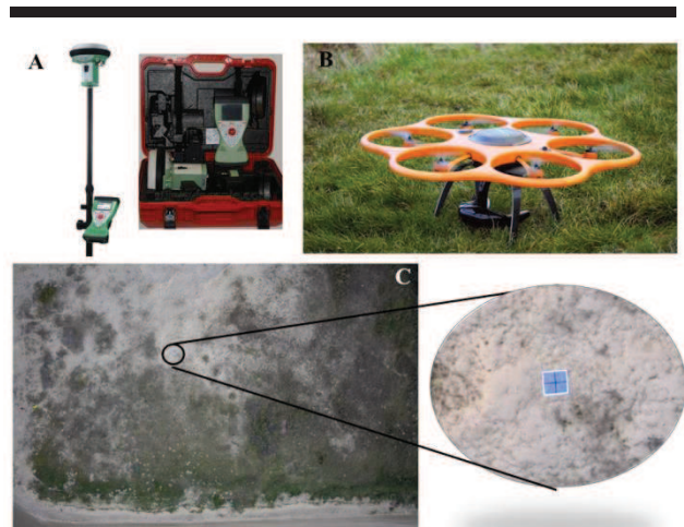
Figure 2. A- GPS-RTK used for the positional accuracy. B – UAV used for data collection. C – GCPs utilized for the positional accuracy.
