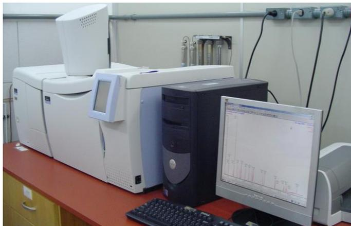
Figura 1. CG-EM Perkin Elmer modelo Clarus 500 MS
