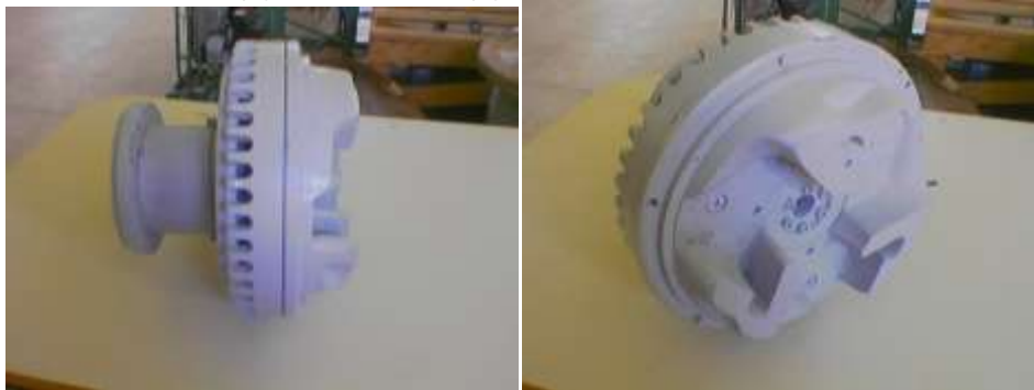
FIGURA 6.1 – Alternador: (a) vista lateral, (b) vista frontal
