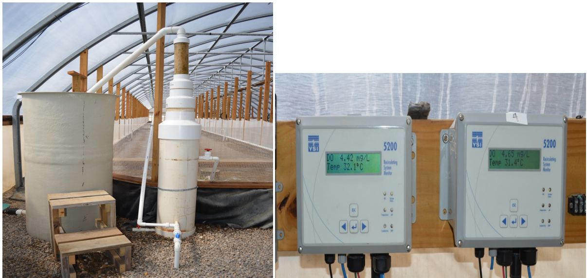
Figure 2. Home-made foam fractionator and DO monitors.
